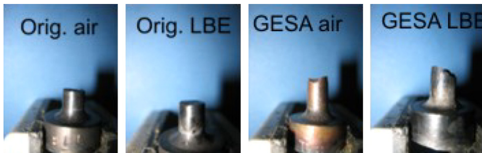
Fig. 8. Morphology of surfaces after tested to failure, strain level for all specimens \Delta\epsilon_t/2 = 0.8\% .
